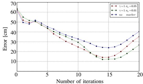
Fig. 3: Case 5a - Average localization error with and without reflective markers, and for different values of  $\gamma$  and  $\sigma_b$ . The marker is visible until iteration 15 approximatively.
