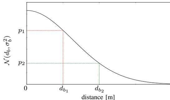
Fig. 1: In the second update step, a new coefficient is computed if markers are detected. The smaller the distance, the more likely the measurement is.
